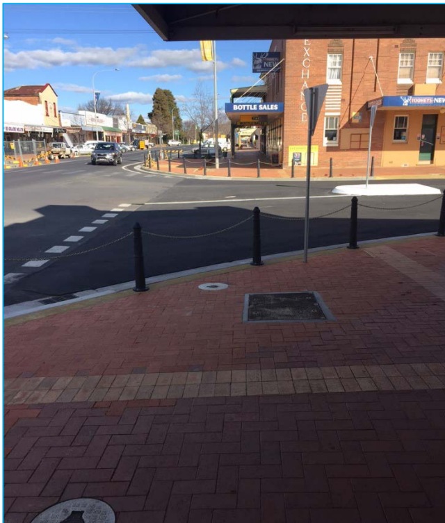
Figure 4-1: The new Adelaide Street / Ogilvy Street intersection crossing diverts pedestrian from their desired path, and creates a (literal) barrier to walking
